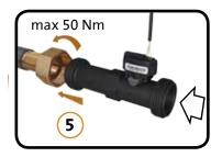
Connect the energy metering device  $(\overline{\mathbf{5}})$  with the pipe via the threaded connector
